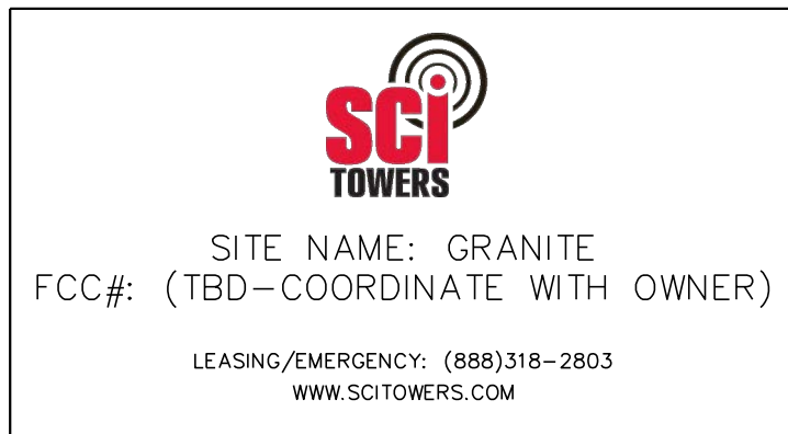
① SCI TOWERS LLC AND FCC REGISTRATION SIGN SIZE: 12"X 24" (0.063" ALUMINUM) (TO BE MOUNTED ON GATE)
