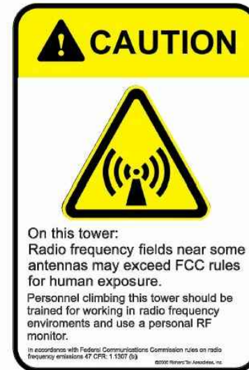
③ RF WARNING SIGN SIZE: 18"X 12" (0.040" ALUMINUM) (TO BE MOUNTED ON GATE)
