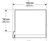
Note 1: All height dimensions include the compressed base insulation sheet (9.0 mm(0.35 in.)).
