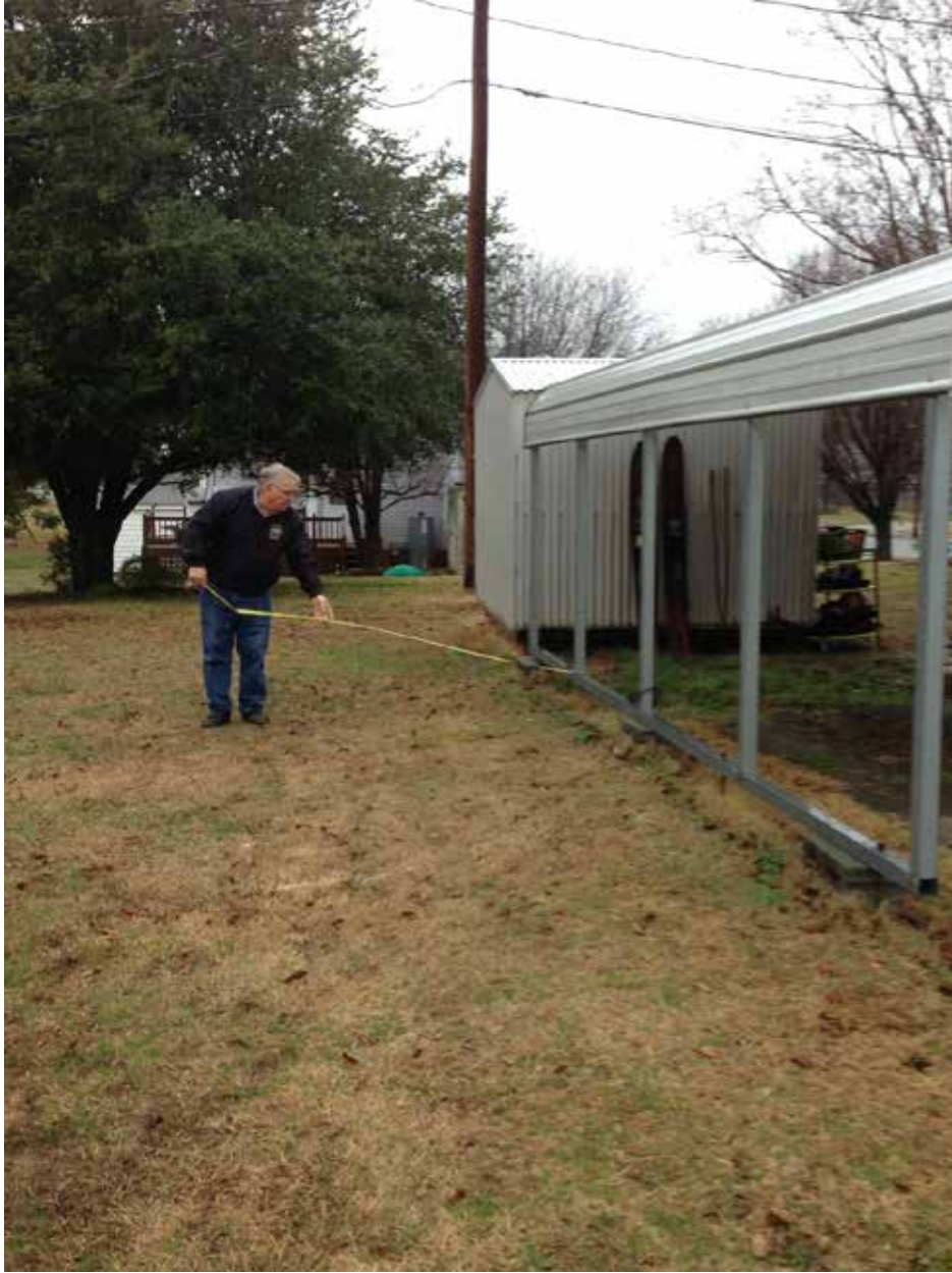
Picture J-3. Harold Kernodle, City of Graham Building Inspector, uses a tape measure to measure the distance from the metal carport to what he has identified as the side property line.
