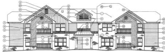
1-14 FRONT ELEVATION - BUILDING TYPE "B" 1/8" = 1'
