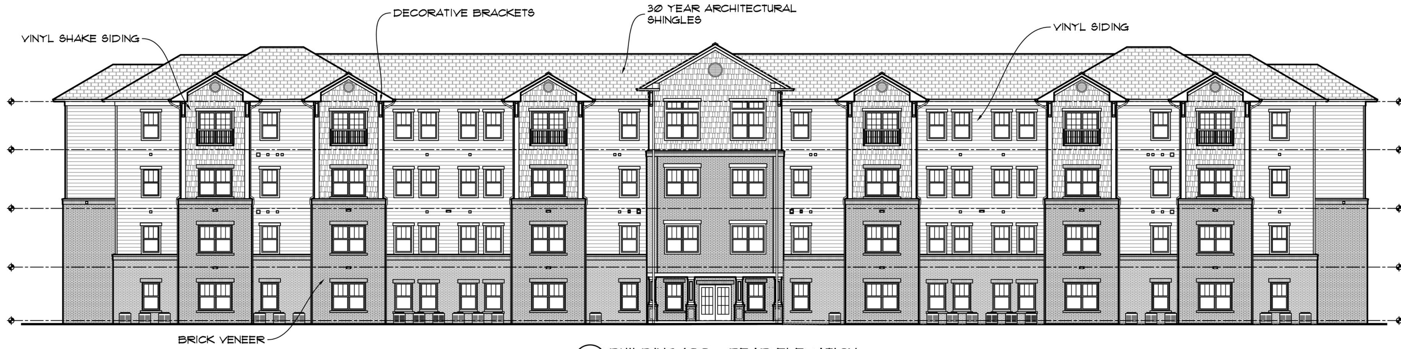
4 BUILDING 100 - REAR ELEVATION 3/32" = 1'-0"
