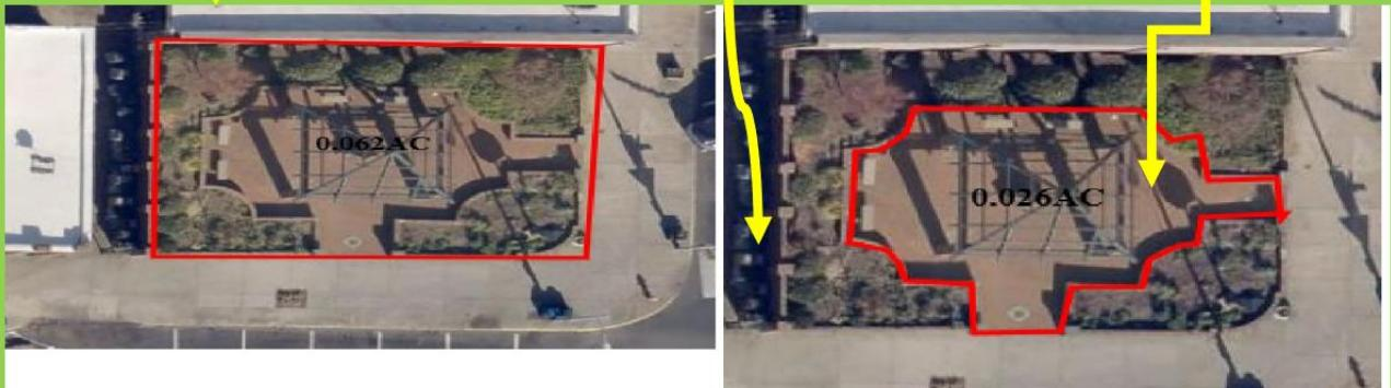
To repair the park in the current condition, it will require a total demolition. Then excavation down to a depth of approximately 9 to 15 feet to reach solid ground. This calculates to removing 40,000 to 55,000 cubic feet of dirt, debris and in-fill. Then transporting the material to a certified landfill location.(approximately 2,500 ton)
