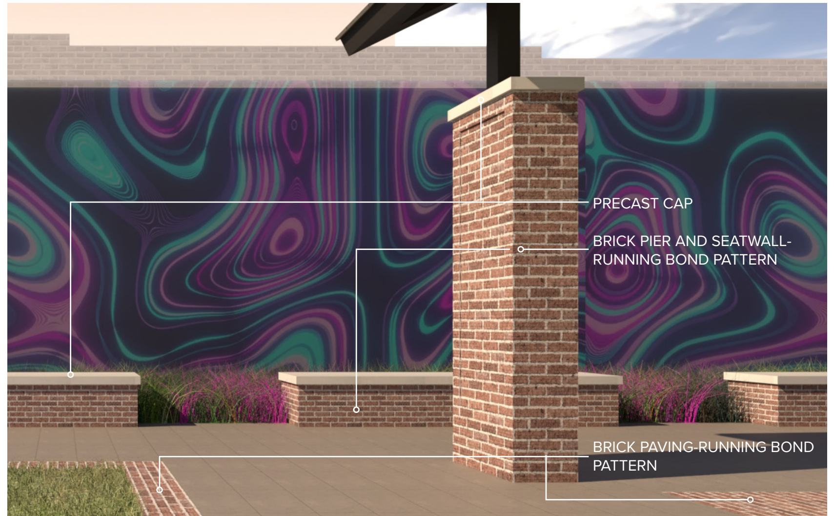
BRICK ELEMENTS OF THE PARK INCLUDE PAVING, PAVILION AND SEAT-WALLS WITH PRECAST CAP
